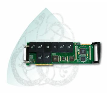
Balder-8U-PCI 8 Access ISDN BRI U-Interface PCI Adapter
