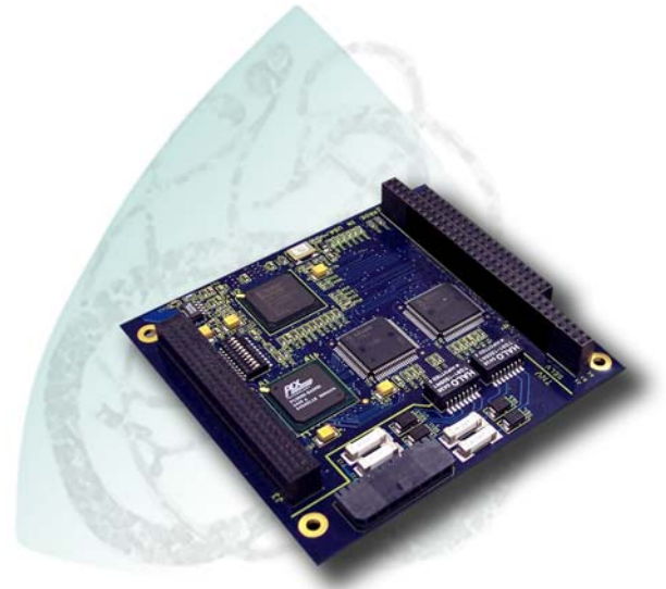
Sleipnir-1-PC104-Plus Adapter for T1/E1 access in the PC104 form factor
