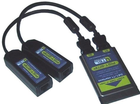
The PCMCIA and PCI cards are supporting both SS7, BICC, V5 and ISDN PRA software modules for protocol analysis and simulation.
