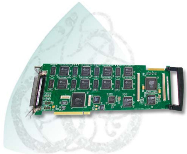
Vidar-5x16-PCI Resource Board
